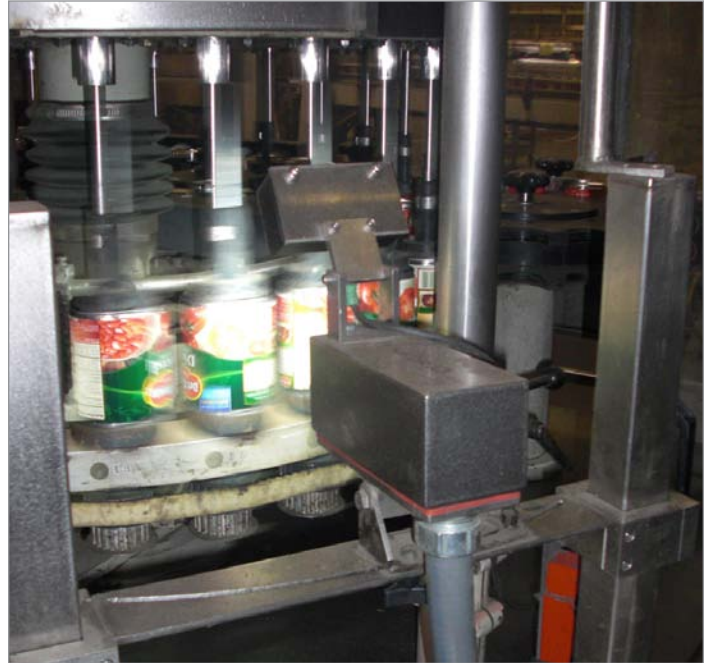
A camera reads the UPC code during the labeling process.
