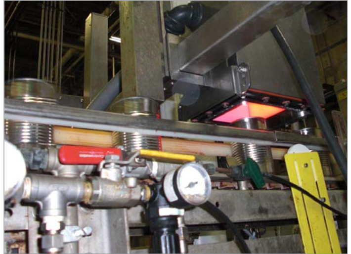
An enclosed camera positioned on a can seamer reads the variety code on the top of the cans.
